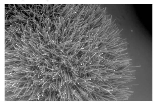
The tip of the applicator of another test stick – FLOQSwabs – was coated with short nylon fibers arranged vertically.
