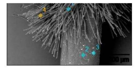
According to the analysis by Professor Gatti, the small white dots on the picture of the swab neck are silver nanoparticles – "Silver is a material that is not declared in the manufacturer's data sheet."
