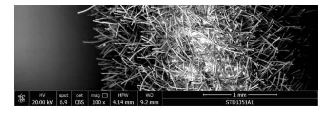
Another swab from Biocomma appeared to be made of fiberglass, or at least to have a fiberglass coating. Components were carbon, oxygen, aluminum, silicon and titanium. It could not be ruled out that an additional coating was made of organic materials.
