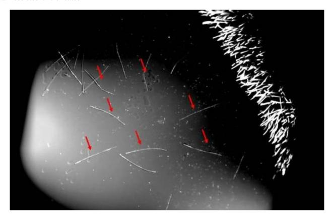
A brush-like test stick from Manta, China, showed a large number of broken fibers. Carbon, oxygen, silicon, zirconium, sulfur, aluminum, titanium and sodium were found to be components of the sample.
